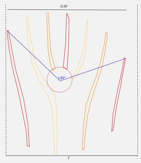
c) We track the rotation of any arbitrary blade, the easiest being the red blade from its top left position to its top right position. This corresponds with a  $600^{\circ}$  rotation (one may be tempted to say a  $240^{\circ}$  rotation but note that the red blade can be seen when the scanning line is at the middle meaning at that point it has already passed the  $240^{\circ}$  mark.
