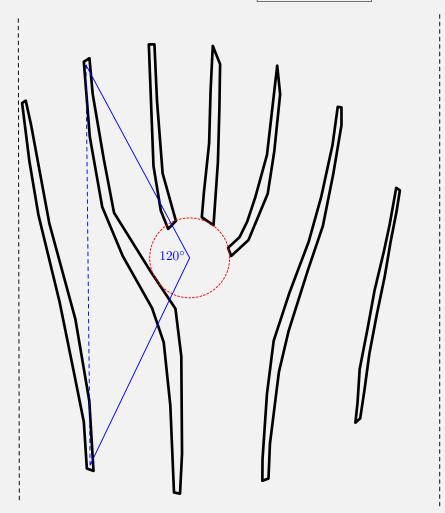
**b)** Refer to the diagram above. The figure shows one column with a maximum of 2 blades on top at a time. If there were 2 blades, only one blade should appear at a time. The blades themselves are marked in black on the figure. It is seen that the angle between the blades is near 120°. Using our assumption that they are equally spaced, this implies a 3-blade propeller.
